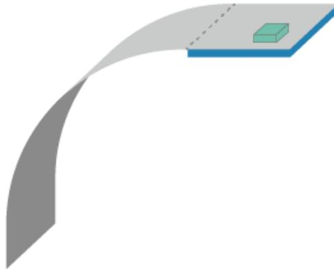
**Figure 10–2 Example of a bend with ample margins so as to prevent folding on the stiffener’ s edges**
