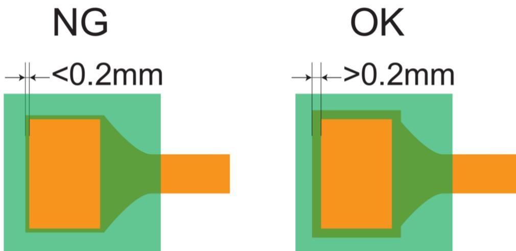
Figure 5-1 Soldermask opening on the inside of copper patterns
