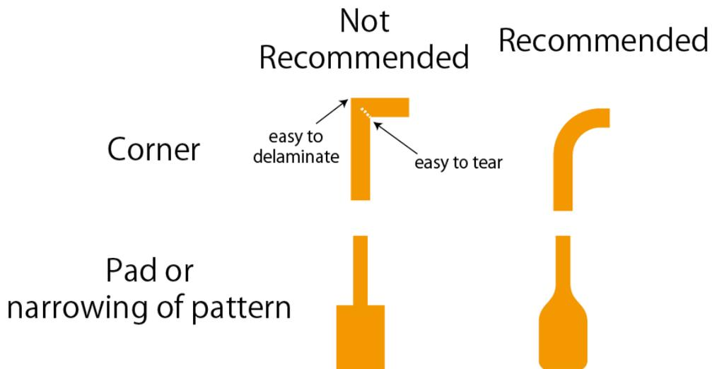
Figure 4-1 Good and bad examples of the shape for corners in wiring and parts of variable wiring width and land
