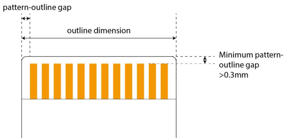
**Figure 8-1** Connector part dimensions
