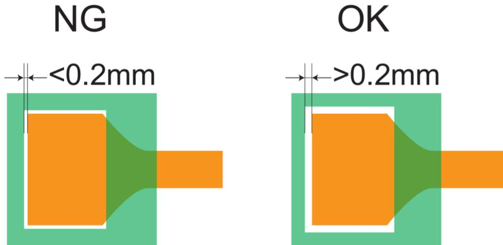
Figure 5-2 Soldermask openings on the outside of copper patterns
